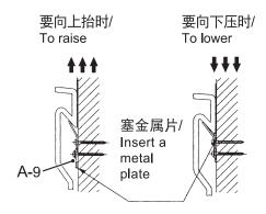
端子台盖板的安装方法/ Terminal block cover installation method
