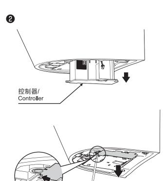
控制器无法降下时,请使用平头螺丝刀将其拆下/ If the controller does not slide out on its own, use a flat-head screwdriver to lower it.
