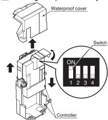
Remove the waterproof cover. Slide the controller up.
