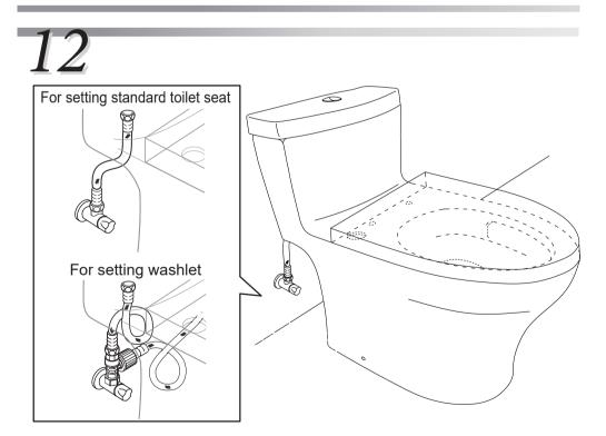
After conducting a test run, confirm that no connections are leaking water. Not installing the product properly may cause water leaks that could result in flooding damage to property, such as household belongings.
