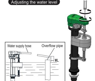
Adjust using a flat-head screwdriver
