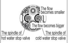
The flow of both hot water stop valve and cold water stop valve reduces during rotating clockwise and increases during rotating anticlockwise. Attention: When turning the water stop valve spindle anticlockwise, take care to use appropriate force. Otherwise, the water stop valve may be removed entirely resulting in water
