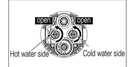
Filter net cleaning when clean the filter net. Please turn off cold and hot water supply valve then use a sleeve wrench to remove the check valve in anti clockwise direction.Clean the filter net after carry out the check valve.
