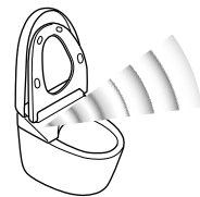
Body sensor B (Detects a person standing in front of the bowl unit.)
